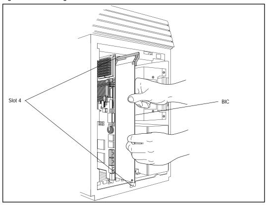
Figure 17 Re-installing the BIC in a new NAM
